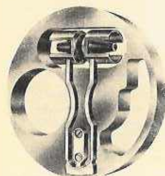
Figure 4. Tuning fork with magnetic iron cups is mounted on movement plate.
