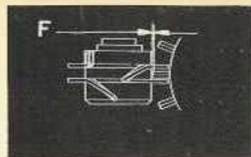
FIGURE 112 illustrates the need for precision adjustments to assure adequate clearance between pallets and escape teeth.
