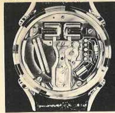
Figure 7. Enlargement of dial side of movement shows electronic circuit at right, tuning fork at center of photo.
