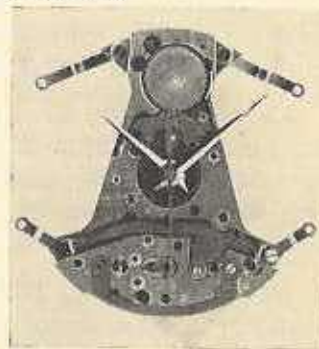
Figure 13. The dial side of the movement without the batteries and battery receptacles. The minute wheel teeth are bevelled for easy meshing with the arbor's hand-setting wheel.
