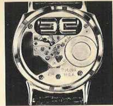
Figure 8. Train-side view shows tiny mercury battery as circle at right, the tuning fork cups and coils at top.
