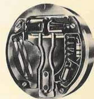
Figure 5. Spacing of magnetic cups at tip of fork around tiny electro-magnets is shown in this cross-section.
