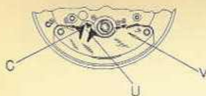
FIGURE 22. In dismantling watch, never try to take apart magnet C , lower shunt bridge V or magnet U which positions the index wheel.
